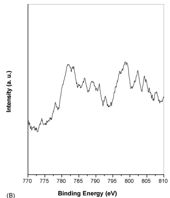
Fig. 7. XPS spectra of (A): (a) Co-MCM-41 (100) and (b) Co-MCM-41 (50); [B] Co/MCM-41 (2).
